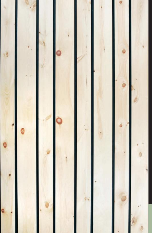
NELMA's Eastern White Pine grade rules define the limiting characteristics (knots, holes, splits, etc.) allowed in each grade (quality level). While the rules describe the poorest piece permitted within a grade, it is unlikely the maximum size or number of these characteristics would be present in any board.
