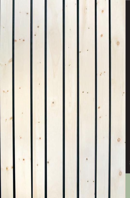
NELMA's Eastern White Pine grade rules define the limiting characteristics (knots, holes, splits, etc.) allowed in each grade (quality level). While the rules describe the poorest piece permitted within a grade, it is unlikely the maximum size or number of these characteristics would be present in any board.
