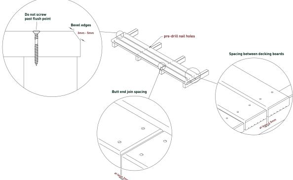
Ensure screws are installed correctly as screw install diagram. In particular, do not over screw past the flush point with the decking and also ensure screws are installed straight (not on an angle as this puts undue pressure on the timber). Remember that KeyDeck is kiln dried and will swell slightly so therefore there is no need to fix the screws past flush with the top of the board! (warranty requirement)
